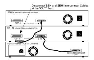
Figure 3-2. Disconnecting the HubSTACK Interconnect Cable
